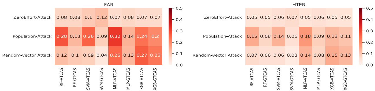
Fig. 4. The performance of V-TCAS and G-TCAS under different adversarial scenarios. The benefit of including Genuine and Impostor-GANs in the pipeline, i.e., G-TCAS architecture, is evident as it consistently achieves lower FARs (in turn HTERs) across the classification algorithms and attack scenarios compared to V-TCAS (the architecture without the two GANs).
